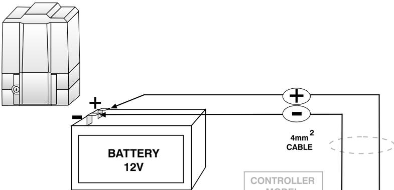
**NOTE: IF A LARGE BATTERY IS USED, THE CABLES CONNECTING THE BATTERY TO THE CP80 CARD SHOULD BE BETWEEN 6 & 10 mm<sup>2</sup> FOR CABLE LENGTHS LESS THAN 5 METRES.**
