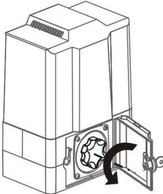
**ROTATE THUMBWHEEL ANTI - CLOCKWISE
