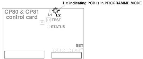
**STEP 2** Hold TEST P/B DOWN until LED L 1, flashes the required number of times as shown in TABLE 5.1, then release P/B.
