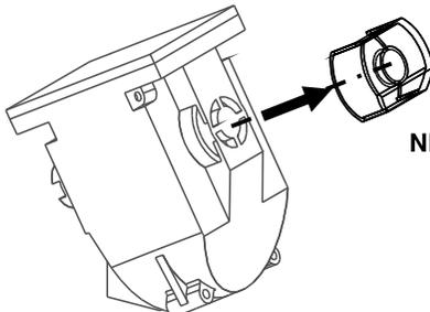
**NB** - Do not throw away the cap, it must be replaced after setting the DOSS.
