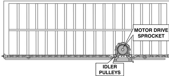
NOTE: Mount chain under idler pulleys and over motor drive sprocket
