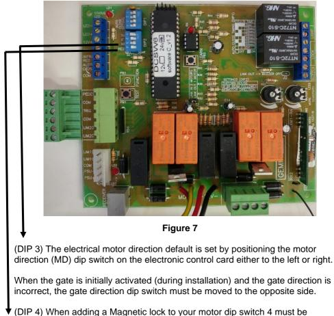
(DIP 4) When adding a Magnetic lock to your motor dip switch 4 must be activated to ensure that the Slave motor opens first upon activation and closes last.
