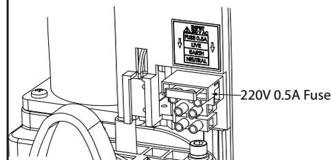
Replace the 0.5A 220V fast blow fuse here.
