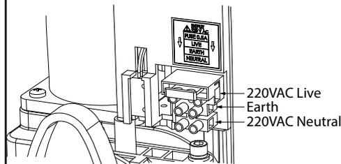
Terminate the 220Vac and earth as shown here.
